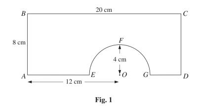
A model bridge is made from a uniform rectangular board, ABCD, with a semicircular section, EFG, removed. O is the mid-point of EG. AB = 8 cm, BC = 20 cm, AO = 12 cm and the radius of the semicircle is 4 cm (see Fig. 1).
