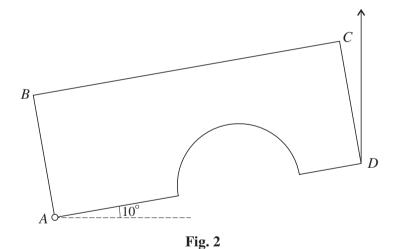
The model bridge is smoothly pivoted at *A* and is supported in equilibrium by a vertical wire attached to *D*. The weight of the model is 15 N and *AD* makes an angle of  $10^{\circ}$  with the horizontal (see Fig. 2). Calculate the tension in the wire. [5]
